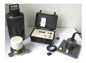
Figure 1: LEMI-018 system with various sensors magnetometer.
